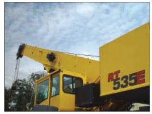
The RT535E incorporates a rectangular boom shape made from 100k.s.i. steel which eliminates weight and improves capacity compared to conventional shapes.
